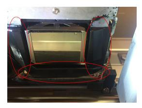
Because of ink Mist and Static Electricity, the black, protective plastic areas around the Print Heads will collect ink and fibers.
