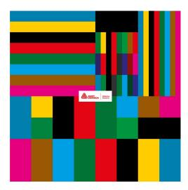
Your TrafficJet printer is an eco-solvent based printer. Printing all colors and channels ensures that ink is flowing through the lines and through the nozzles which will reduce the natural tendency of ink to collect and solidify in the nozzles. Instituting a policy to print regularly will help maintain your TrafficJet printer and reduce maintenance costs.
