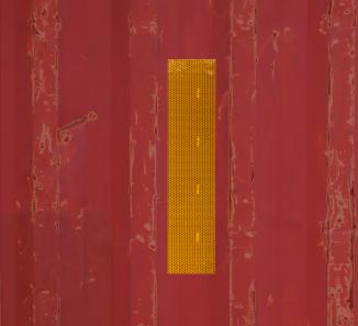
Retroreflective conspicuity tape on the sides of railcars improves motorist safety at railroad crossings.
